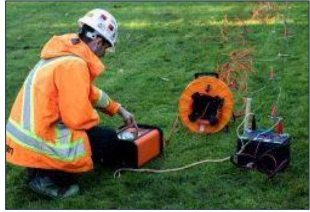
Seismic refraction (hammer and monitoring equipment) Electrical resistivity monitoring equipment.
