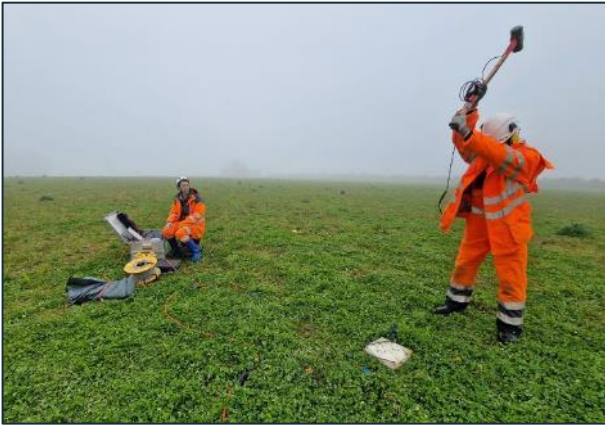
Seismic refraction (hammer and monitoring equipment) Electrical resistivity monitoring equipment.
